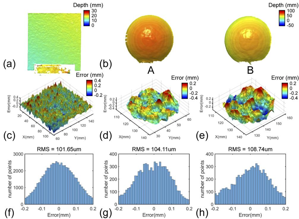
**Fig. 7.** Precision analysis for measuring a ceramic plane and a pair of standard ceramic spheres using our method. (a) The 3D reconstruction results of a ceramic plane, (b) the 3D reconstruction results of a pair of standard ceramic spheres, (c)-(e) the corresponding distributions of the measured errors of (a)-(b), and (f)-(h) the corresponding quantitative histograms of the measured errors of (a)-(b).
