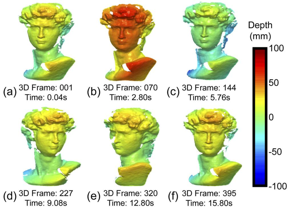
**Fig. 9.** The 3D reconstruction results for a dynamic scene: a moving David model ([Visualization 1](#)). (a)-(c) The David model moves along the Z axis and (d)-(f) the David model rotates around the Y axis.
