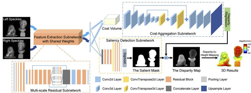
**Fig. 3.** The schematic diagram of the proposed end-to-end stereo matching network. The whole stereo matching network is composed of a multi-scale residual subnetwork (as the shared feature extraction subnetwork), construction of the 4D cost volume, cost aggregation using 3D convolutional layers, disparity regression, and a saliency detection subnetwork.
