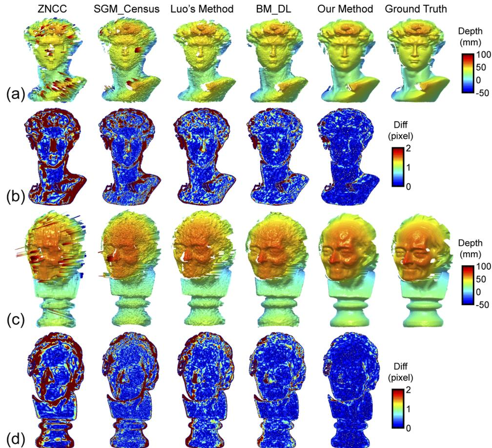
**Fig. 6.** Comparison of the 3D reconstruction results using different methods. (a) the 3D reconstruction results of the David model, (b) the matching errors of the David model, (c) the 3D reconstruction results of the statue of Voltaire, (d) the matching errors of the statue of Voltaire.
