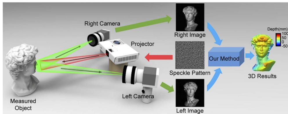
**Fig. 1.** The diagram of the proposed single-shot 3D shape measurement method using an end-to-end stereo matching network for speckle projection profilometry.
