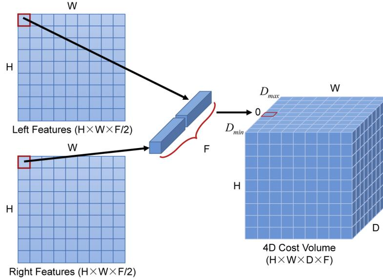
**Fig. 4.** The schematic diagram of the construction of the 4D cost volume. Based on the disparity range of our SPP system, the initial 4D cost volume is built by combining feature tensors of each pixel in the left image and all corresponding candidates along the epipolar line of the right image.
