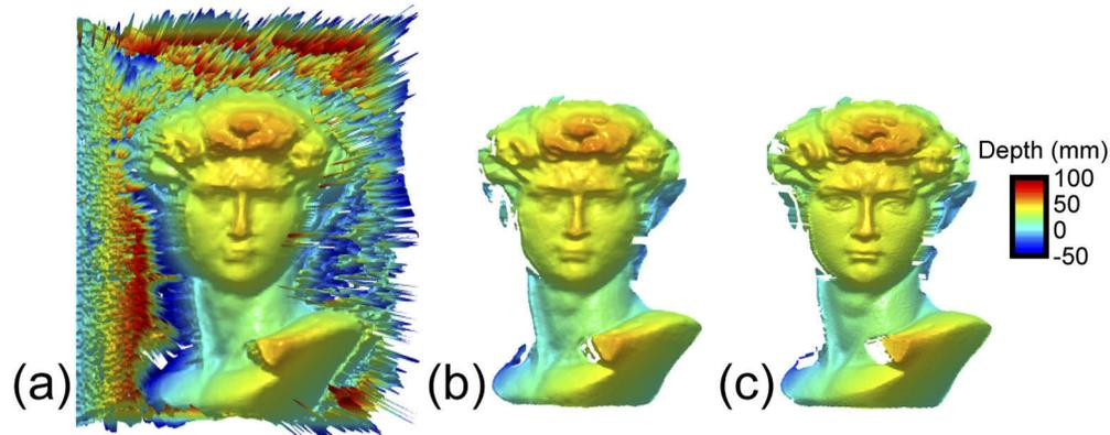
**Fig. 5.** Comparison of the 3D reconstruction results without/with the saliency detection network. (a) the 3D reconstruction results without the saliency detection network. (b) the 3D reconstruction results with the saliency detection network. (c) the ground truth.
