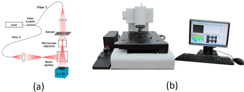
Figure 11. The Michelson-structure digital holoscope. (a) Optical configuration. (b) Packaged system.
