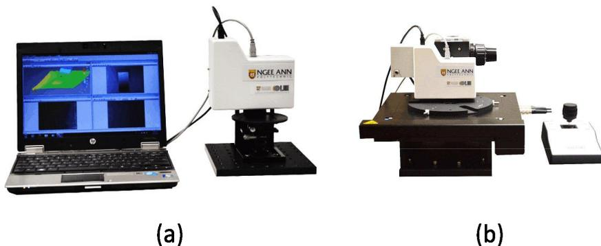
Figure 9. The compact digital holoscope with the built-in laser (a), and a motorized stage (b).
