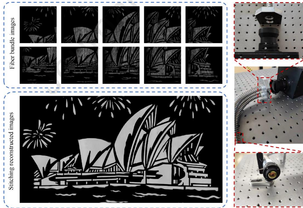
Fig. 7. Stitching results based on the fiber bundle and corresponding sub-eye images.
