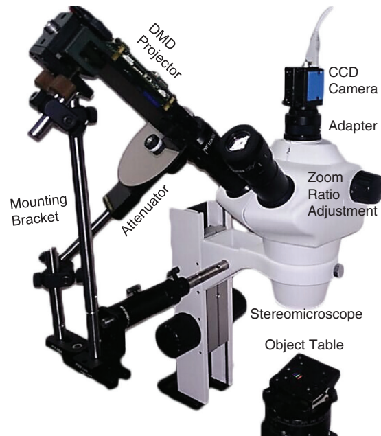
Figure 2. Physical map of our micro-3D surface profile measurement system based on a Greenough-type stereomicroscope.
