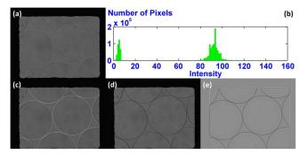
Fig. 7. Experimentally captured intensity at focus (a) with its histogram (b), and the intensity at  $-550 \ \mu m$  (c) and  $+550 \ \mu m$  (d) as well as their intensity derivative  $\partial I/\partial z$  (e).
