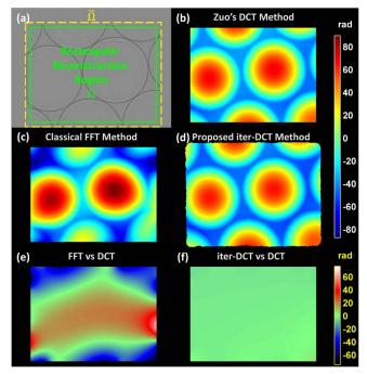
Fig. 8. Zuo's DCT method uses the information in "data region  $\overline{\Omega}$ " to retrieve phase in reconstruct region  $\Omega$  (a), and its result (b) is used as a benchmark to judge the results from classical FFT-based TIE solver (c) and the result from the proposed iter-DCT method (d). The phase retrieved with the proposed method is much closer to the DCT result (f) than the FFT one is (e).
