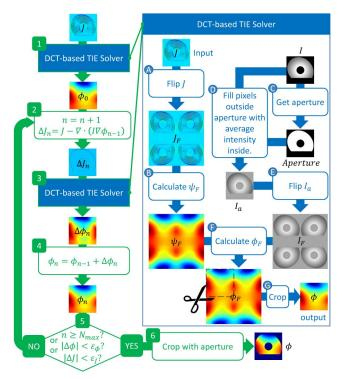
Fig. 2. Iter-DCT-based TIE solver is illustrated for phase retrieval with an arbitrarily shaped hard aperture.
