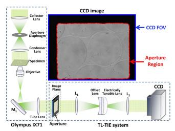
Fig. 6. TIE experiment is implemented by using an inverted bright-field microscope and a tunable lens-based TIE module with placing an aperture at the image plane.
