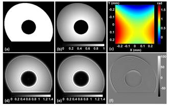
Fig. 3. TIE through a hard aperture, (a) which is in an irregular shape, (b) is simulated with calculated intensity at focus, (c) true phase, (d) calculated intensity at z = -0.5 mm and (e) z = 0.5 mm, and (f)  $\partial I / \partial z$ .
