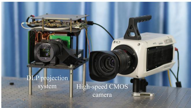
Fig. 8. This system includes a high-speed CMOS camera and a DLP projection system.
